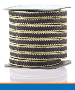
CHAMPION KOMBIFLON™ Style 176 is a Combination Packing with tough para aramid fibre yarn (with each strand impregnated with PTFE dispersion and lubricated with Silicone oil) cross-plaited at the corners, ePTFE and graphite fibre yarn at
